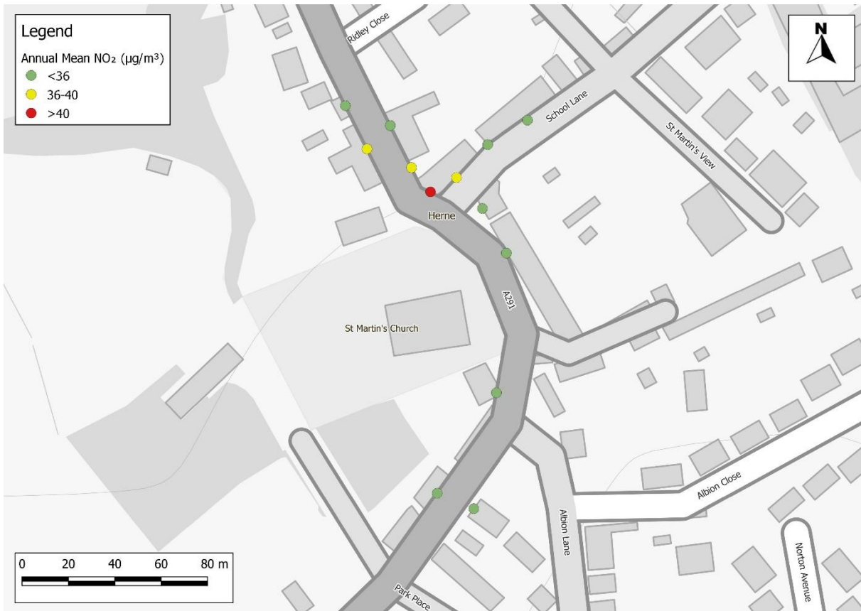
Figure 2: Modelled Annual Mean NO 2 Concentrations at Specific Receptors in 2022 Baseline in Herne
